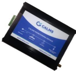
CALMS-EDGE-0 survey device LTE 4G with Modbus RTU & TCP/IP;
